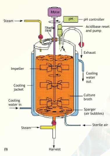
Fig. 3. Basic features of a fermentor (Bioreactor).
