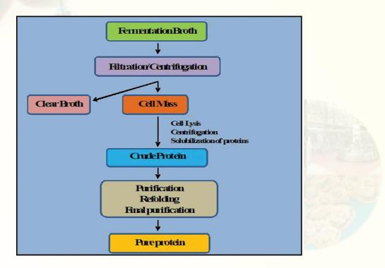
Fig. 10. Isolation of an intracellular microbial product (clear broth is discarded). Example: Recombinant insulin (Humulin®) from *E. coli*.
