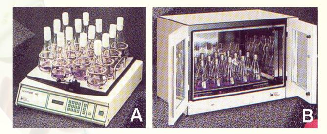
Fig. 2. (A) Shaker; (B) Incubator Shaker.
