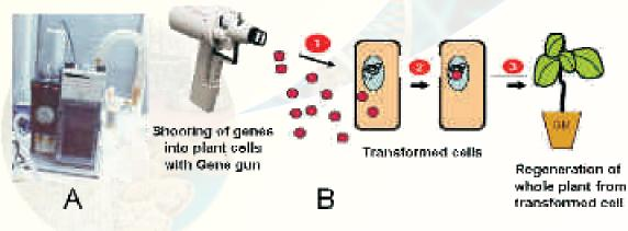
**Fig. 8.** The Bio-rad Gene gun machine, Model He1000 (A), and the schematic diagram showing the bombardment of gold particles containing the DNA (gene of interest) on their surface onto the plant cells in culture to produce transgenic plants with desirable traits (B).
